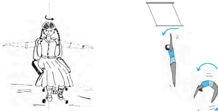
Fig. 6.32: (a) Conservation of angular momentum on a swivel chair. (b) An acrobat using the principle
