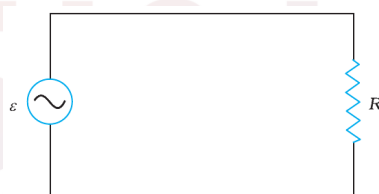
Fig. 7.1: AC voltage applied to a resistor
